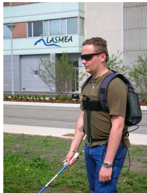
Figure 1 Synoptic of the vision based localization system (left) and the pedestrian prototype with a chest mounted camera and a wearable computer in a back pack (right).
